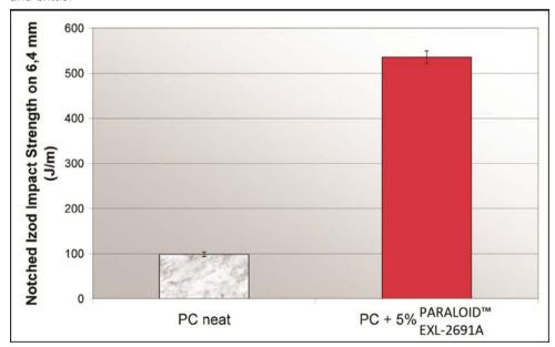
In binary blends such as PC/ABS, the primary core-shell particles of the PARALOID™ EXL-2691A Impact Modifier preferentially locate at the interface between both phases improving their compatibility. This results in improved welding line properties and improved heat stability.
