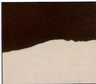
Figure 8 - Black tread compound contains the nonstaining antiozonant DURAZONE 37.
