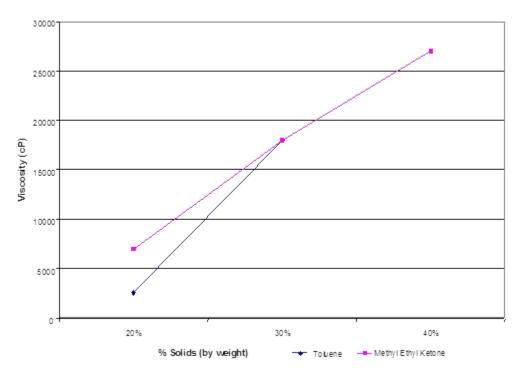
Viscosity of Elvacite(r) 2041 in Solution
