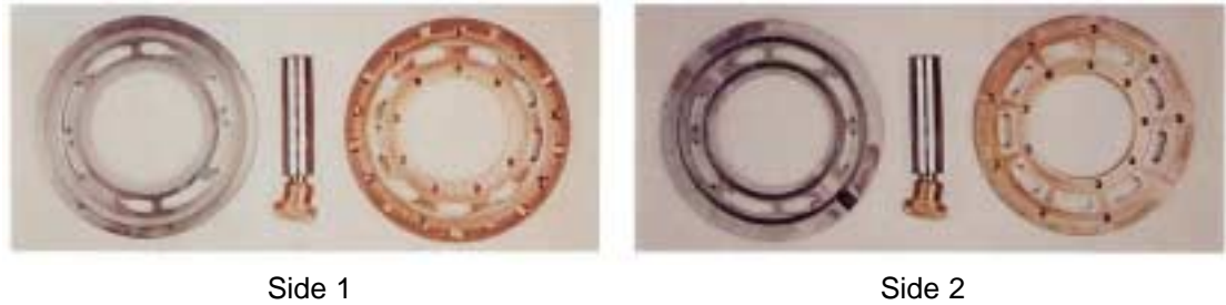
Figure 2 • Sunstrand Series 22 Axial Piston Pump Parts After Running 225 hr with UCON® Hydrolube HP-5046D
