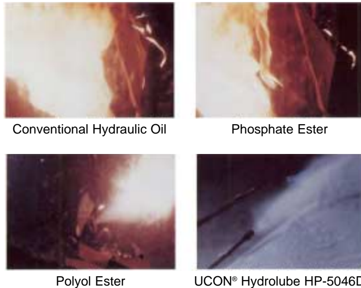
Figure 3 • Spray Flammability Testing of Various Hydraulic Fluids
