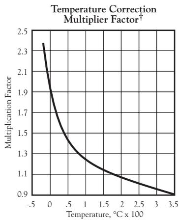
†Note: Below 40°C, an error in the temperature correction factor above 5% may be incurred. This is dependent on the diameter and velocity effect on the Reynolds number and friction factor.
