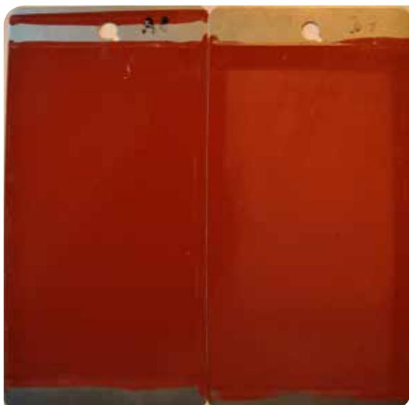
Fig 2. Appearance of primer after 300 hours of QUV ageing
