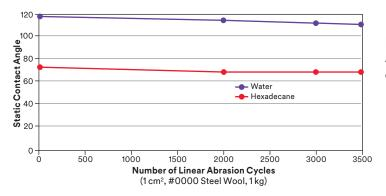
Even after abrasion with steel wool, the Static Contact Angle remains stable. Contact angles are correlated to easy clean capabilities.
